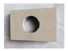
Where the cut face will be visible inside the hole, a PCD tipped hole saw for concrete produces a smoother finished face, but will be slower, and greater care is needed to prevent breakout of the back of the board.
