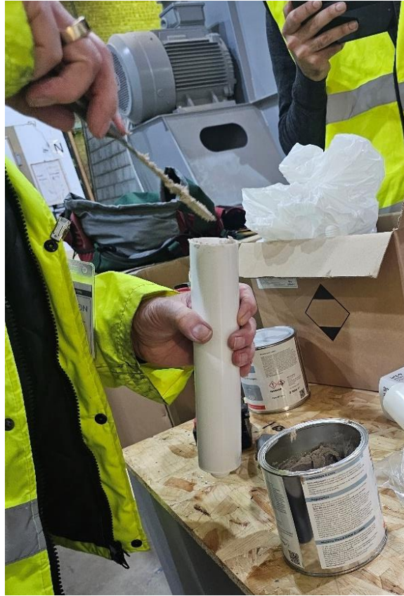
Plate 13 – Mixed Adhesive Transferred into a Plastic Tube
